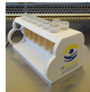
Magnetic separation rack can hold 12 standard microtubes
